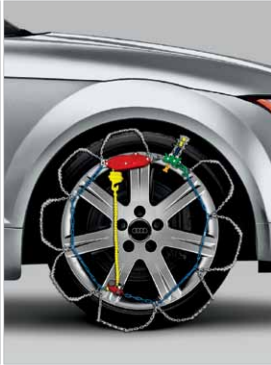
Snow chains 1 Snow chains made of case-hardened alloy steel on a spring steel hoop are easy to mount and dismount. Check local regulations prior to use. Ask your authorized Audi Dealer about compatibility with your vehicle and wheels.
