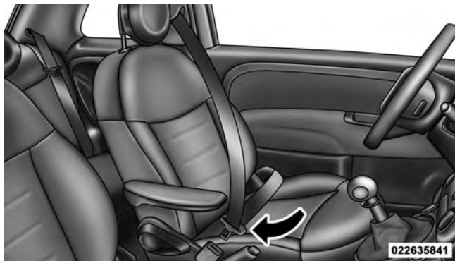
Inserting Latch Plate Into Buckle
