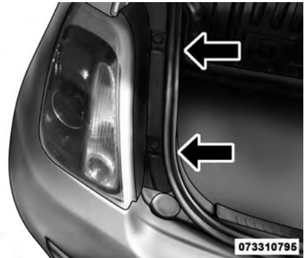
Tail Lamp Assembly Screws
