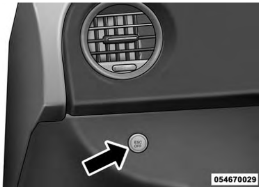
ESC Off Switch (Manual Transmission)
