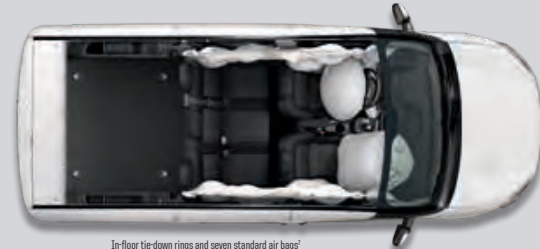
In-floor tie-down rings and seven standard air bags 7
