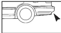
4. The inside of the rear bumper can trap dirt and salt. Rinse it out occasionally.
