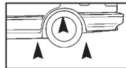
3. Dirt and salt tend to build up on control arm pivot mounts. A blast from your garden hose will keep them clear.
