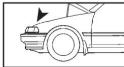
5. Spray the radiator fins from the back side to rinse away salt and sand that may accumulate in the radiator fins.
