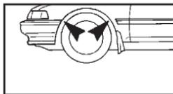
2. Wash the inside of the front and rear wheelhousings to prevent dirt and salt build-up.
