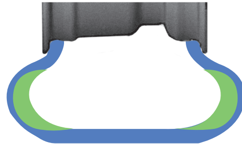
BMW Approved Run-Flat Tire and EH2+ wheel after a puncture
