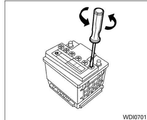
1. Remove the battery vent caps with a screwdriver as shown.
