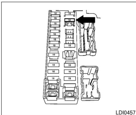
If a type A fuse is used to replace a type B fuse, the type A fuse will not be level with the fuse pocket as shown in the illustration. This will not affect the performance of the fuse. Make sure the fuse is installed in the fuse box securely.
