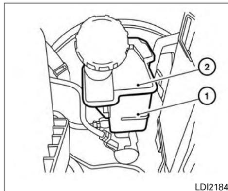
Check the fluid level in the reservoir. If the level is below the MIN line ①, add Genuine NISSAN Super Heavy Duty Brake Fluid or equivalent DOT 3 fluid up to the MAX line ②. If fluid must be added frequently, the system should be checked by a NISSAN dealer.
