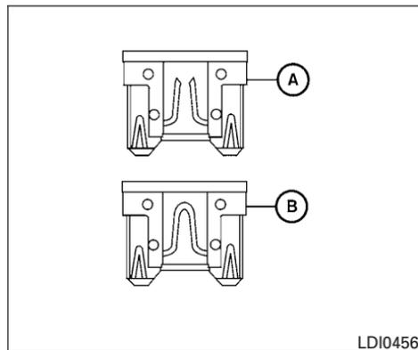
5. If the fuse is open (A), replace it with an equivalent good fuse (B).
