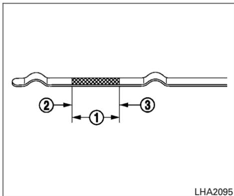
5. Remove the dipstick again and check the oil level. It should be between the H (High) and L (Low) marks ①. This is the normal operating oil level range. If the oil level is below the L (Low) mark ②, remove the oil filler cap and pour recommended oil through the opening. **Do not overfill** ③.
