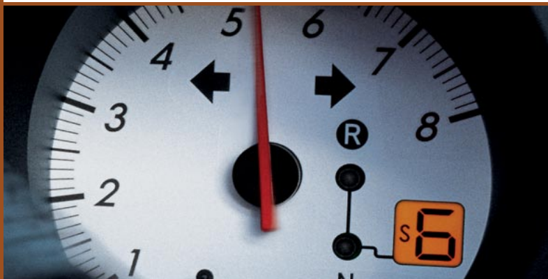
6-speed sequential manual transmission tachometer.
