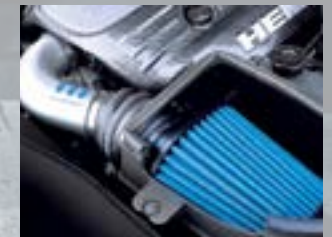
COLD AIR INTAKE SYSTEM
