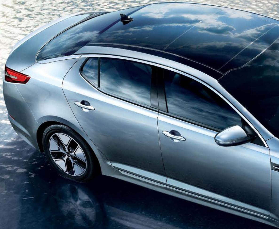
**HYBRID** It's not your ordinary hybrid midsize sedan. The 2012 Optima Hybrid delivers class-leading<sup>9</sup> horsepower of 206 total (electric motor and gas engine) and highway fuel efficiency of 40 mpg.<sup>3</sup> All thanks to the electric motor, a lighter and more powerful lithium polymer battery, regenerative braking, reduced engine friction, electric-powered air conditioning and aerodynamic styling.
