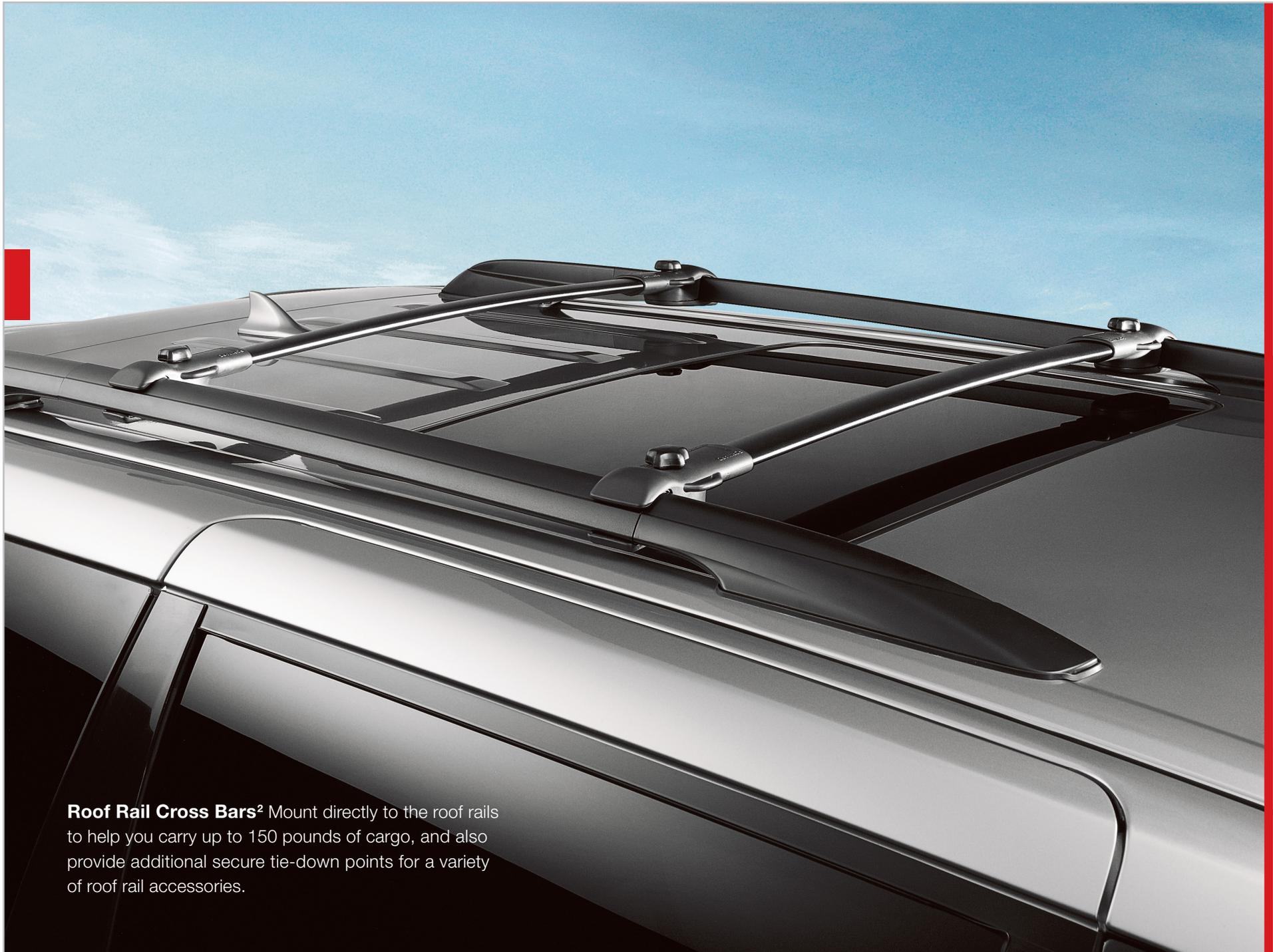
**Roof Rail Cross Bars<sup>2</sup>** Mount directly to the roof rails to help you carry up to 150 pounds of cargo, and also provide additional secure tie-down points for a variety of roof rail accessories.
