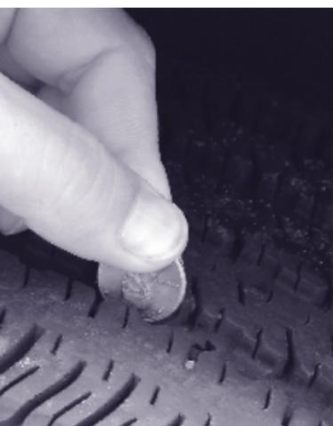
When they appear “even” with the outside of the tread, it is time to replace your tires. Another method for checking tread depth is to place a penny in the tread with Lincoln’s head upside down and facing you. If you can see the top of Lincoln’s head, you are ready for new tires.
