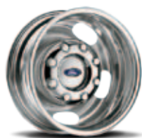
17" Polished Forged-Aluminum Standard: F-350 DRW/F-450
