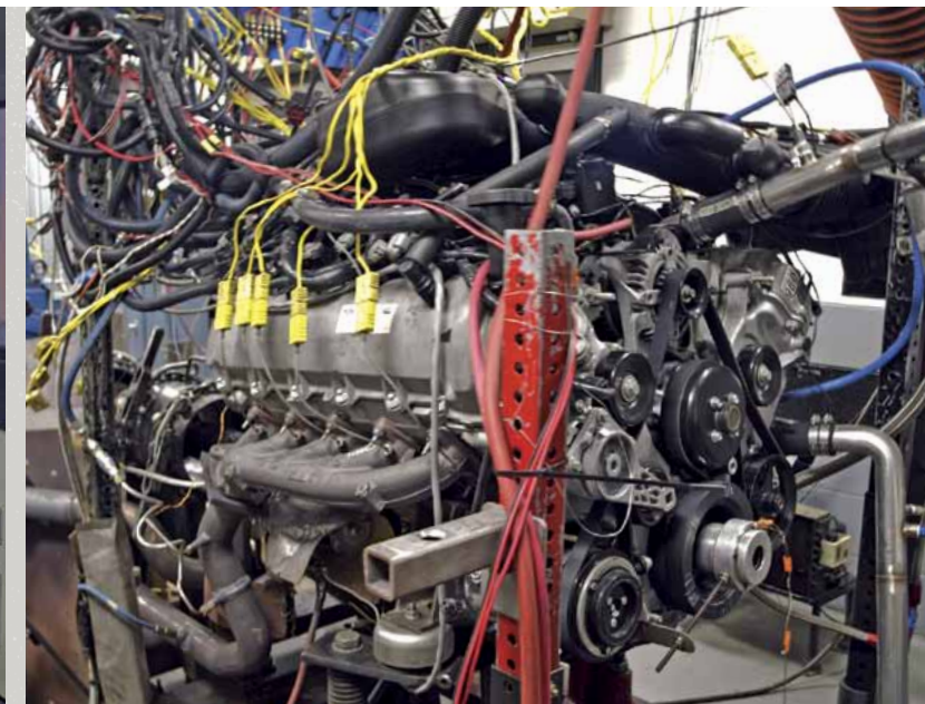
Engine dynamometer and calibration tests. 6.8L V10 engine shown.
