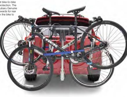
To avoid blocking taillights, use only roof mounted bike carriers to transport bikes with solid disc wheels. Before installing this carrier, please check the laws of your state regarding license plate visibility.
