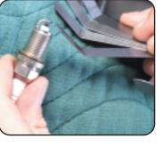
INSTALL SPARK PLUGS – Be sure that each new spark plug has a new metal washer. Install each plug as far as possible by hand. Make sure the plug is correctly threaded. Tighten firmly with the spark plug wrench or socket but DO NOT OVER-TIGHTEN. See the repair manual for proper torque specification.
