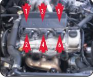
V8 (2VZ-FE) – When facing the engine with the drive belts closest to you, the left side of the engine has cylinders 2-4-6-8. The right side has cylinders 1-3-5-7.
