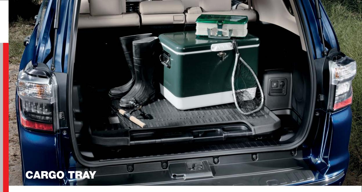
Go ahead, throw those muddy boots in the cargo area. The carpet will still be pristine thanks to this cargo tray<sup>4</sup>, molded from a tough, flexible polymer blend that can be pulled out and hosed off.
