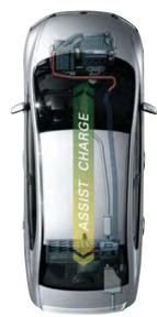
Civic Hybrid's 1.3L i-VTEC® engine operates in tandem with a lightweight, high-output selfcharging electric motor for extra fuel efficient power when needed. In some instances, the Hybrid can cruise on the electric motor alone.
