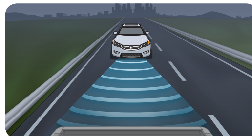
ADAPTIVE CRUISE CONTROL (ACC)¹¹ ACC electronically regulates your following distance in Adaptive Cruise Control mode, accelerating or decelerating depending on how close you are to the vehicle detected in front of you. (Touring)
