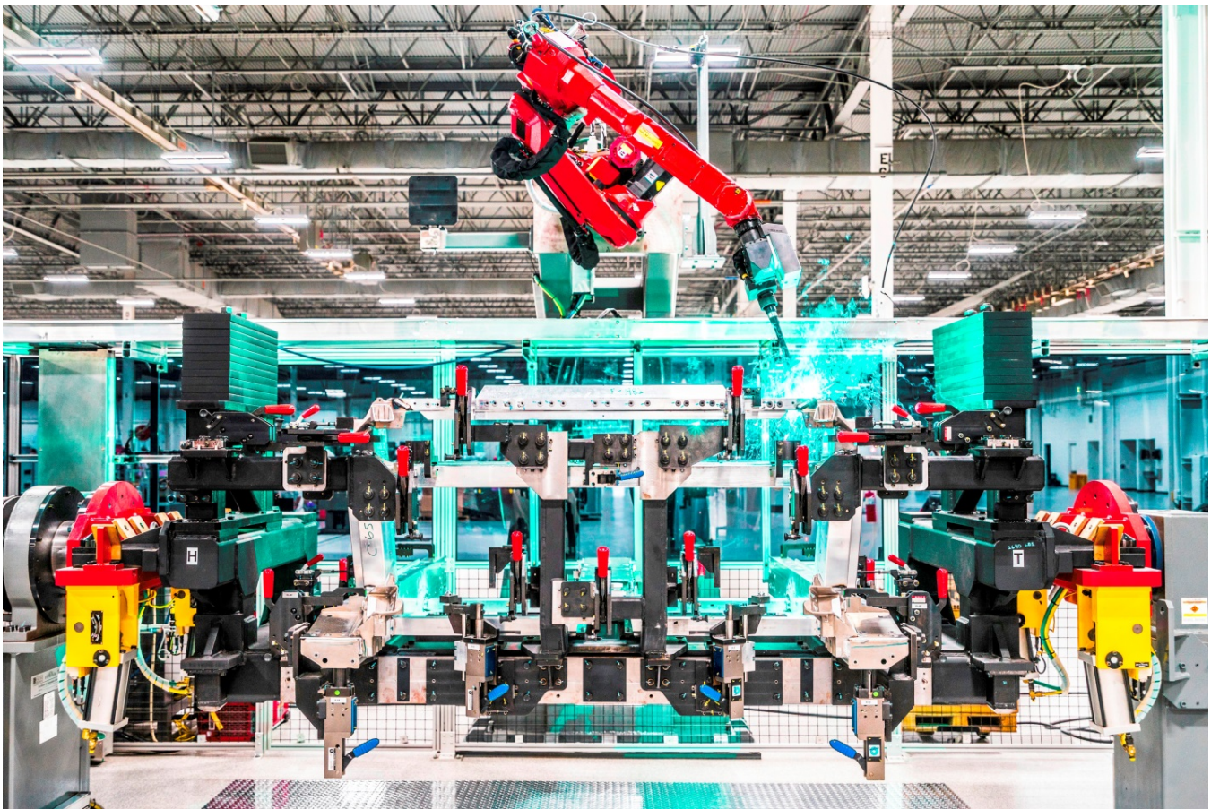
NSX space frame construction at the Performance Manufacturing Center
