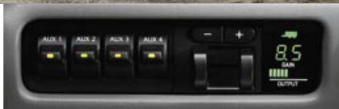
Trailer Brake Controller shown to the right of Upfitter Switches, which are standard on F-350/F-450/F-550 Chassis Cab; optional on F-250/F-350 Pickup (66S).
