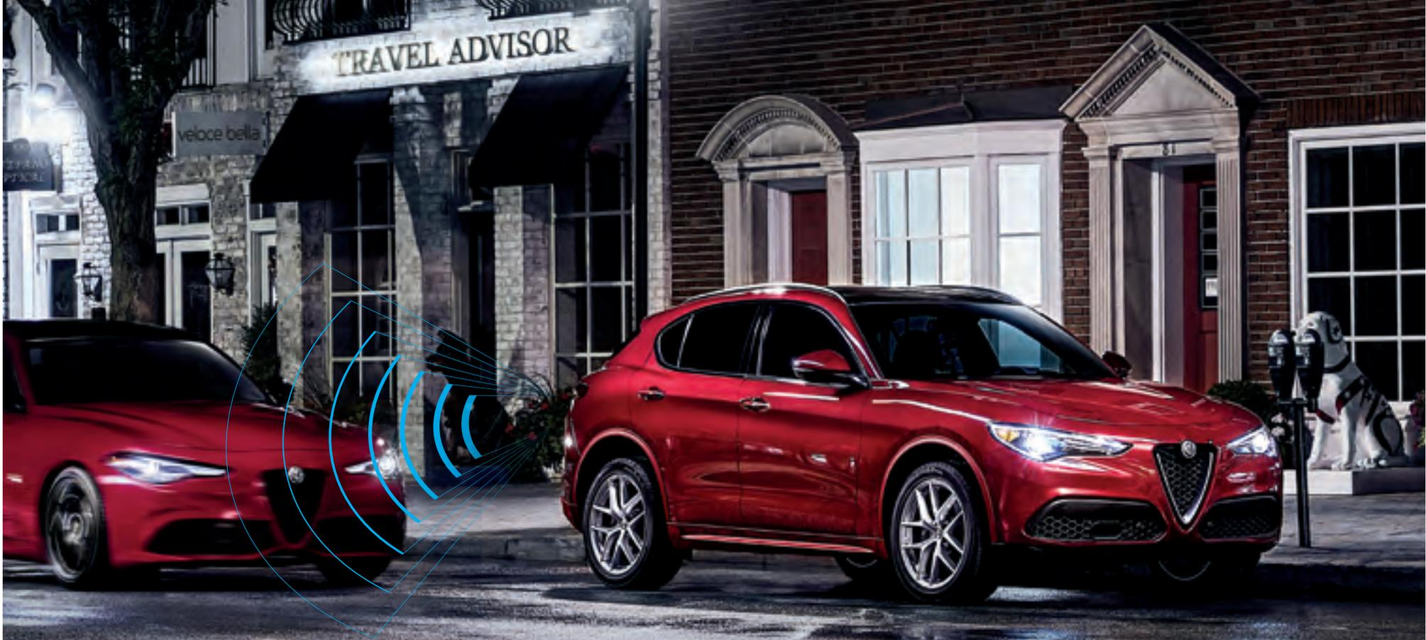
**BLIND SPOT MONITORING (BSM)<sup>5</sup>** This available system has dual ultra-wideband radar sensors that aid the driver when changing lanes, and when trailing vehicles are in the blind spot, via an illuminated sideview mirror icon (standard on Quadrifoglio).
