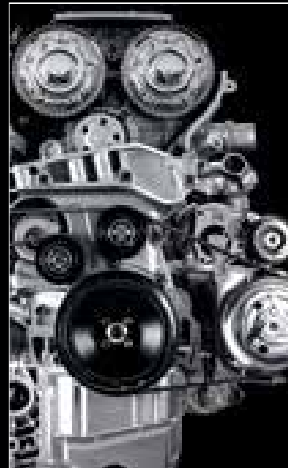
1750 turbocharged, aluminum, 4-cylinder engine
