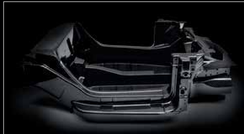
Genuine carbon fiber monocoque chassis
