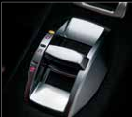
4-position, Alfa DNA driving mode selector
