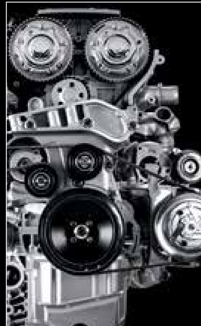
1750 turbocharged, aluminum, 4-cylinder engine
