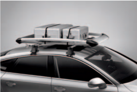
Ski and snowboard racks 1 Push-button, keyed locks open and close easily. Rubber-cushioned aluminum bars hold securely. Standard attachment (shown) holds two sets of skis or two snowboards. Deluxe attachment holds up to three sets of skis or four snowboards.
