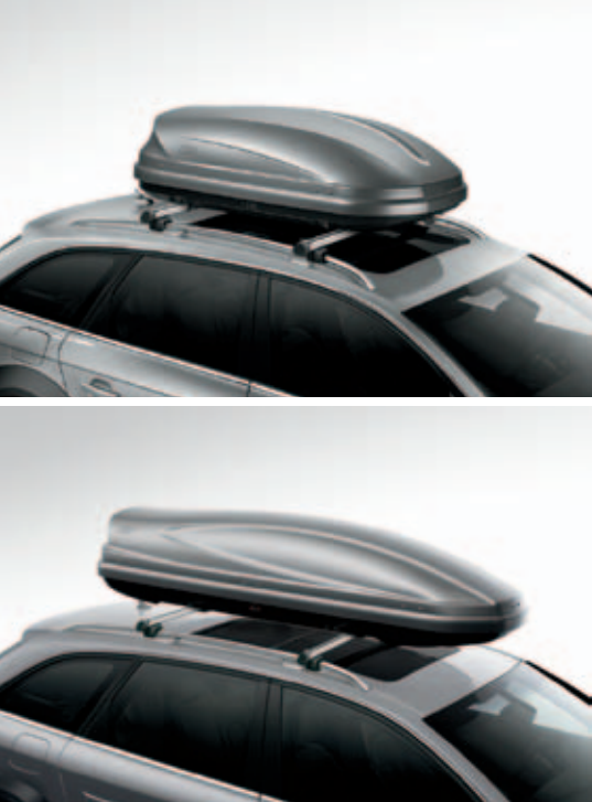
Small cargo carrier Extra carrying capacity (13-cu-ft) comes in a smart size: 55" long, 35" wide, 14" high.
