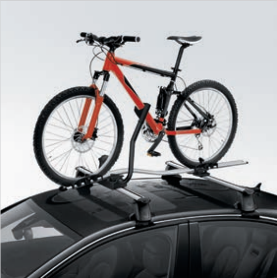
Aluminum bike rack This locking holder fits 20- to 80-mm bike frames with both wheels on the bike and helps keep the bike upright as you secure it in place. 3,4
