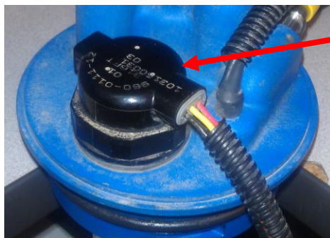
DEF Level Sensor
