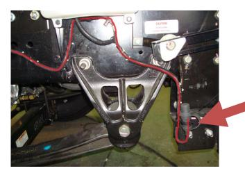
Existing cable assembly 10020987 with non-bumper mounted receptacle connection.
