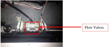
3. Each flow valve has a lock nut to prevent the setting from inadvertently changing. To change the setting, loosen the lock nut, and turn the screw clockwise to slow it down (decrease air pressure) or counter clockwise to speed it up (increase air pressure).
