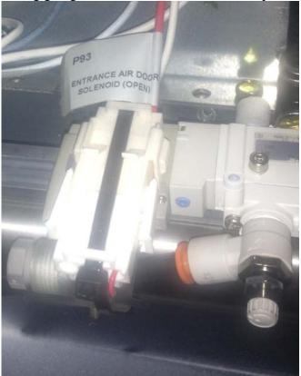
Note: If there is no tag, the open valve is to the left as you are facing it in the bus. The close valve is to the right as you are facing it in the bus.
