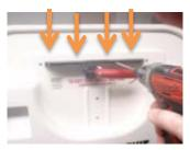
Step 6: Remove the Plastic Receiver and two (2) Anti-rattle springs from the parts kit. Place the two (2) springs in the holes on the back side of the new receiver.
