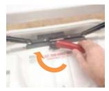
Step 14: Close the lid, guide the metal bracket into the groove on the plastic receiver (as shown in Step 12). Rotate the red handle 90 degrees clockwise to secure the lid (as shown in Step 13). The replacement is complete.
