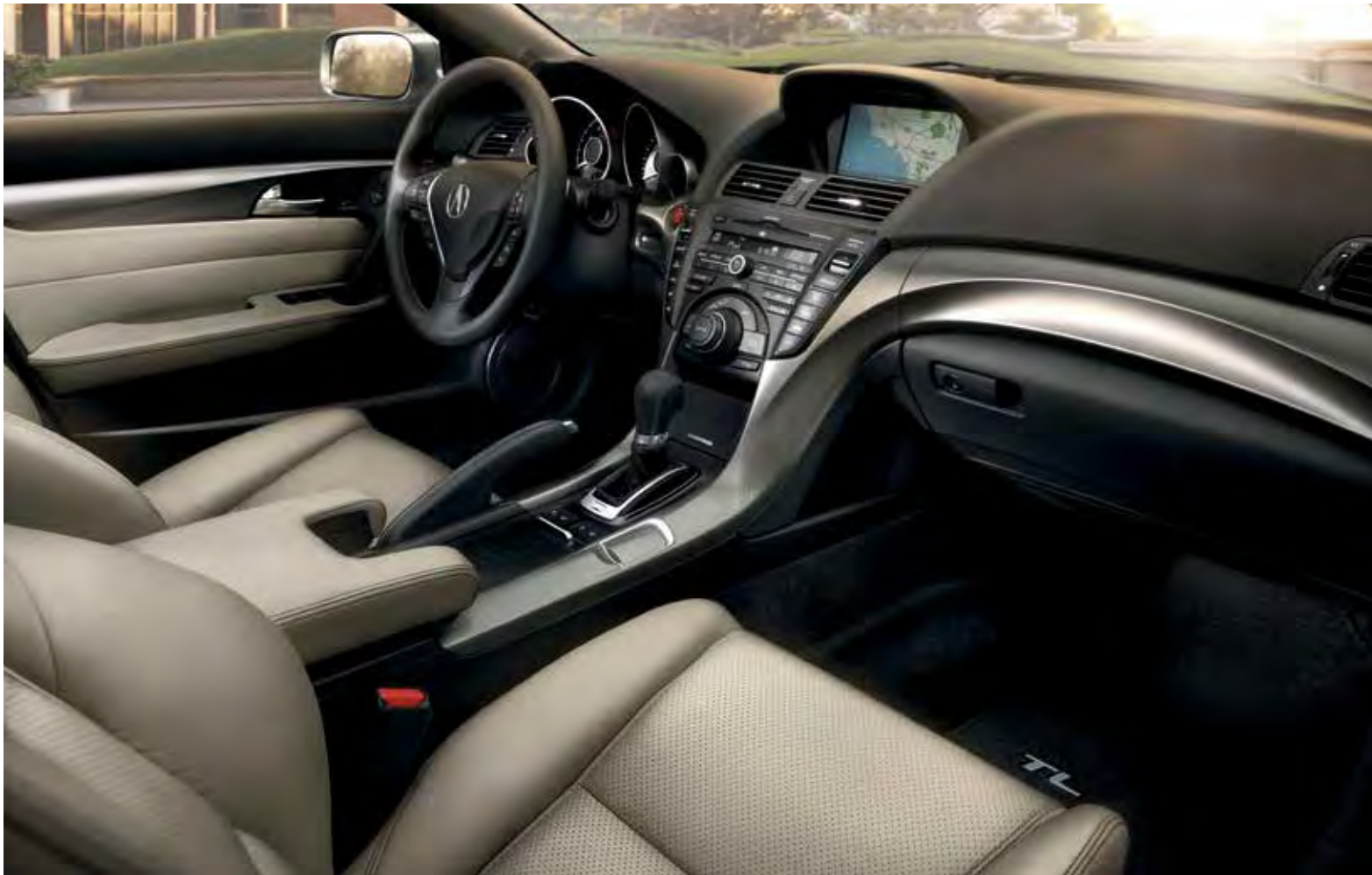
10-WAY POWER DRIVER'S SEAT features a combination of soft and dense materials to help filter out road vibration.
