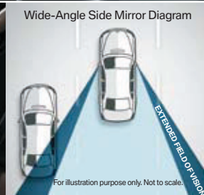
Wide-Angle Side Mirror Diagram
