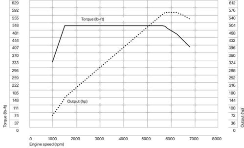
Maximum torque is available across an extremely broad rev band, from 1500 to 5650 rpm, creating rapid responsiveness not normally associated with a turbo engine. Traction is also consistently high, even in the upper rev ranges.
