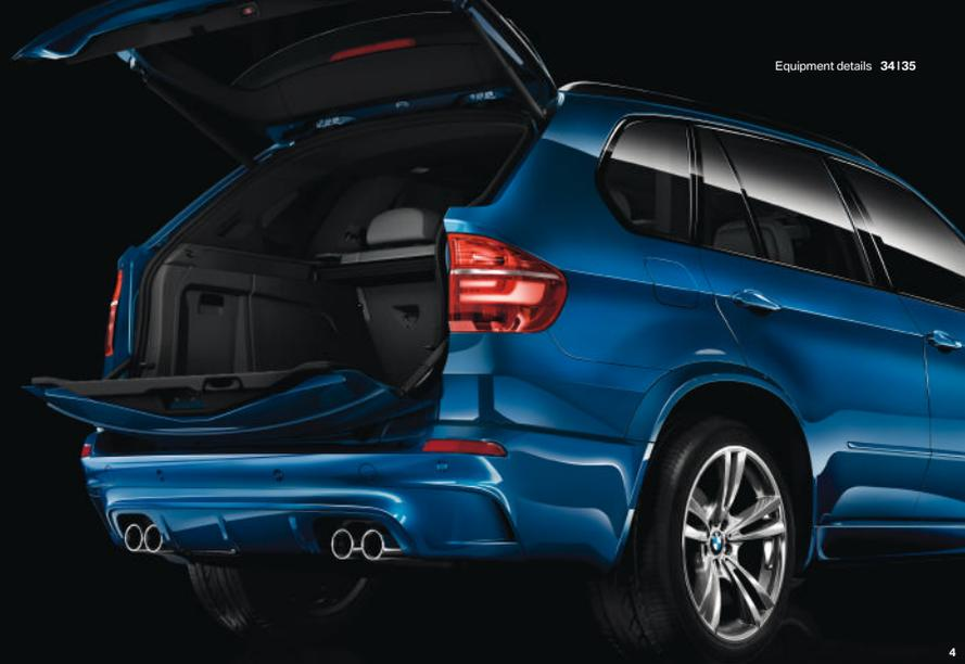
4 X5 M Rear apron with M quad tailpipes; V Spoke (Style 299M) light cast alloy wheels.
