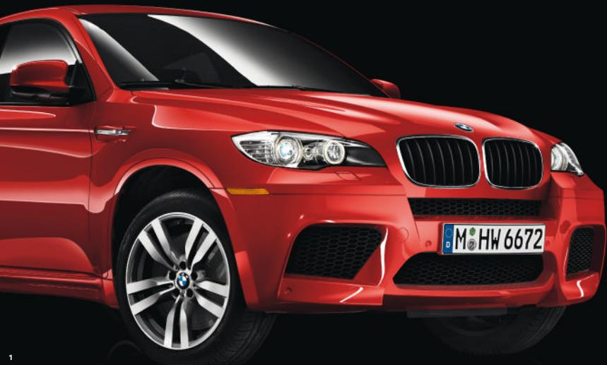
1 X6 M front apron with large air intakes and flaps; Double Spoke (Style 300M) light cast alloy wheels.
