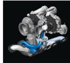
Two highly efficient Twin Scroll turbochargers form the basis of an astonishingly rapid response. A BMW-patented cross-bank exhaust manifold combines the exhaust flows from each of the cylinder pairs (illustration, far left). These are then routed into a channel in the snail-shell-like turbine housings (hence "scroll"), separate from the exhaust flows of the other cylinders, thus enabling them to reach the turbine wheel unimpeded and at high speed (illustration, right).
