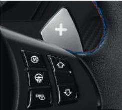
The M Drive function acts as a "memory button" for key driving dynamics, including suspension, stability, steering and throttle sensitivity. Customize these driving dynamics using the iDrive controller by selecting either Normal (default mode) or Sport modes. In addition, Dynamic Stability Control has three modes: Off, Normal and M Dynamic Mode. Once these settings are saved, just press the M Drive button, and they're recalled for driver convenience.
