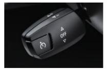
■ Cruise Control lets you store and keep to a chosen speed above 20 mph. It is activated via the left-hand steering column switch and deactivated by applying the brakes or via the switch.<sup>6</sup>
