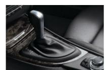
☐ 6-speed STEPTRONIC automatic transmission provides a choice of three modes: "Drive," which incorporates BMW's Adaptive Transmission Control; "Sport" automatic, for a more dynamic shift pattern; and STEPTRONIC automatic, for the hands-on control of a manual without using a clutch.
