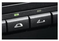
■ Power softtop roof control switch for fully automatic opening and closing of the roof is within arm's reach of the driver and front passenger. Softtop will open and close while traveling at speeds of up to 25 mph.
