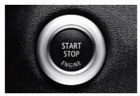
■ Engine Start/Stop button<sup>5</sup> and remote key control the engine. First, insert the remote key into the starter switch slot. After the electronic identification system confirms that it is the correct remote key, you can start (or later, turn off) the engine by pressing the Start/Stop button.
