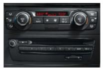
■ Automatic climate control system allows occupants to select a specific cabin temperature and choice of fan speeds, as well as automatic or manual airflow and recirculation. "Convertible" mode also reacts to exterior temperature and sunlight. The automatic recirculation control activates whenever certain air pollutants are detected. The system also includes defrost/demist and MAX A/C functions.
