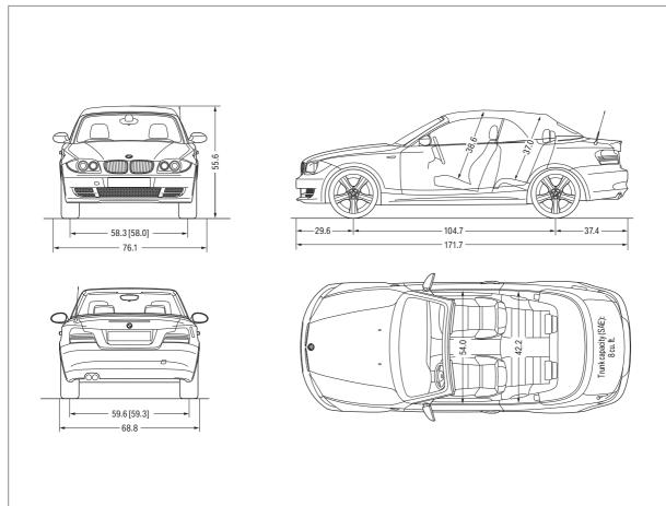
All dimensions are shown in inches, and apply to the 128i with standard wheels. Figures in [ ] refer to 135i.
