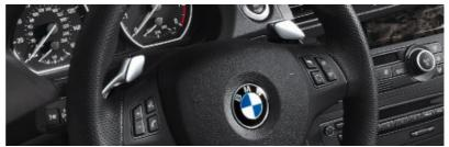
☐ Steering wheel-mounted paddle shifters, shown with the three-spoke, leather-wrapped multi-function M sport steering wheel, allow you to shift gears manually without a clutch. This optional feature comes included in the 1 Series Convertible when it is equipped with optional STEPTRONIC automatic transmission and optional Sport Package.
