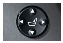
□ Lumbar support for front seats adds four-way power-adjustable comfort for the lower back. Lumbar support can be adjusted up/down and in/out. (included in opt. Premium Package)
