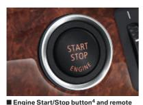
key control the engine. First, insert the remote key into the starter switch slot. After the electronic identification system confirms that it is the correct remote key, you can start (or later, turn off) the engine by pressing the Start/Stop button.
