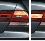
■ Adaptive Brake Lights increase vehicle visibility and signal the intensity of your braking action.
