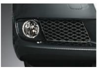
■ Halogen free-form foglights, integrated into the deep front spoiler, enhance your margin of safety in bad visibility. Ellipsoid free-form technology ensures even light distribution on the road.
