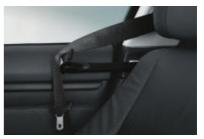
■ Automatic safety belt assistant for the two front seats makes buckling up easier by bringing the belt forward whenever you get into the vehicle. As soon as the safety belt is clicked, the arm retracts into its housing. (If the safety belt for an occupied seat isn't used, the arm retracts after one minute or as soon as the vehicle reaches a speed of about 4 mph.)
