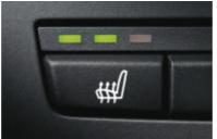
Heated front seats are a welcome feature for driver and front passenger in cooler weather. By pressing the icon button, seat surface and backrest are heated and quickly radiate comfortable warmth in your choice of three settings.
