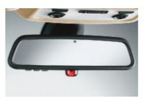
The automatic-dimming inside rear-view mirror darkens in response to the bright headlights of vehicles behind you. The easy-to-read digital compass, integrated into the mirror, is a convenient way to constantly keep your bearings while driving.
