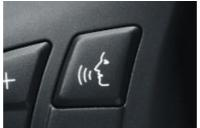
☐ Voice Command allows you to activate numerous Navigation system functions, record up to five minutes of notes, and make phone calls (if so equipped) hands-free. The Voice Command button must be pressed before each use, so conversations won't accidentally activate the phone or other systems.
