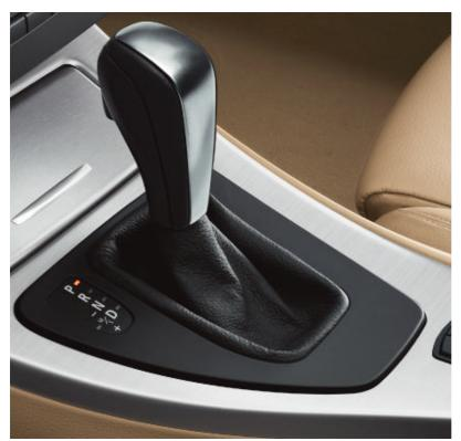
☐ 6-speed STEPTRONIC automatic transmission provides a choice of three modes: "Drive" with Adaptive Transmission Control; a more dynamic "Sport" mode; and STEPTRONIC automatic, for the hands-on control of a manual without a clutch.<sup>1</sup>
