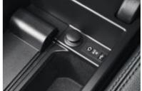
■ Auxiliary input port lets you connect an external audio source, such as an iPod® or MP3 player.
