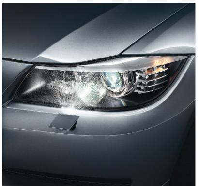
Retractable **high-intensity headlight washers**<sup>1</sup> help keep lights clear of ice, mud, road salt and other coatings, for maximum road lighting and enhanced driving safety.
