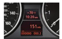
■ The on-board computer with Check Control provides feedback on the vehicle's operating status: oil level indicator and distance to next service appointment/oil change, as well as other detailed information, such as spark plug and micro-filter status. It also provides travel information, including travel range on remaining fuel, external temperature, and more.
