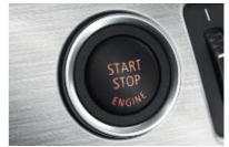
■ Engine Start/Stop button<sup>1</sup> and remote key control the engine. First, insert the remote key into the starter switch slot. After the electronic identification system confirms that it is the correct remote key, you can start (or later, turn off) the engine by pressing the Start/Stop button.
