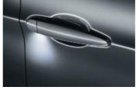
■ Convenient lighting features make it easy to see inside and outside the vehicle. When the door is locked, press the remote's "lock" button to turn on cabin lights and the illuminated door handle. When you open the door, lights shine down to illuminate the ground where you step.
