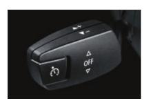
■ Dynamic Cruise Control lets you set and keep to a chosen speed above 20 mph, automatically applying the brakes downhill. It is activated via the left-hand steering column switch, and deactivated by applying the brakes or via the switch.<sup>2</sup>
