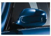
Power-adjustable folding exterior sideview mirrors automatically dim when reflecting bright lights, helping to eliminate glare when driving at night.
