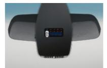
■ Rain sensor measures the amount of rain. In "intermittent" windshield wiper mode, it automatically adjusts the wiping interval as needed. Includes Automatic headlight control (not shown), which activates headlights by means of a sensor that responds to darkness. The rain sensor is also integrated into the braking system as part of the Brake Drying feature.
