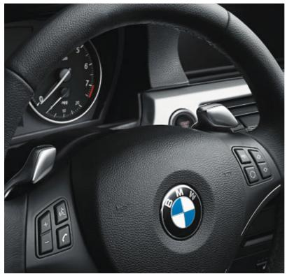
☐ Three-spoke leather-wrapped multi-function sport steering wheel, with steering wheel-mounted paddle shifters that allow you to shift gears manually without using a clutch. This option is included in the 3 Series Sports Wagon when equipped with the optional Sport Package and optional STEPTRONIC automatic transmission.
