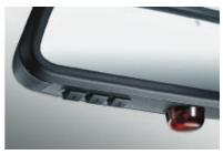
BMW Universal garage-door opener takes the place of up to three remote-control devices. It can activate remote functions outside the vehicle, such as garage-door openers or home-lighting systems.
