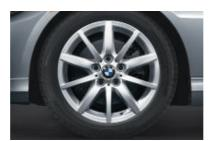
Star Spoke (Style 286) light alloy wheels and run-flat<sup>4</sup> performance tires.<sup>2</sup> In front: 17 x 8.0 wheels and 225/45 tires; in back: 17 x 8.5 wheels and 255/40 tires. (Included in 328i Sport Package; optional in 328i xDrive with Sport Package)
