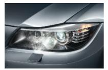
■/□ Retractable high-intensity headlight washers help keep lights clear of ice, mud, road salt and other coatings, for maximum road lighting and enhanced driving safety. (std. in 328i xDrive; included in 328i Cold Weather Package)
