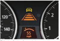
□ Active Cruise Control allows the driver to set a desired speed that is automatically maintained in free-flowing traffic. As a slower-moving vehicle is approached, a radar sensor alerts the system and adjusts speed to match the slower vehicle, while maintaining a preset following distance. As the lane ahead clears, the system automatically returns the car to the set speed.²
