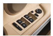
■ Power window buttons with "one-touch" up/down operation and exterior mirror adjustment controls are located conveniently to the left of the driver, allowing access that doesn't require taking your eyes from the road.
