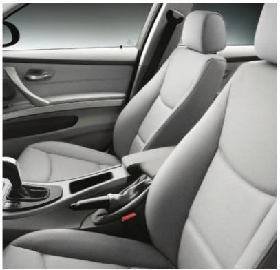
■ Standard front seats, shown here with optional Dakota Leather upholstery, offer 8-way manual adjustment, including 2-way headrests with Active Head Restraints feature. The front passenger seat also includes manual height adjustment.
