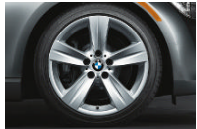
Star Spoke (Style 189) light alloy wheels and run-flat 2 performance tires. 3 In front: 18 x 8.0 wheels and 225/40 tires; in back: 18 x 8.5 wheels and 255/35 tires. (335i Sport Package)
