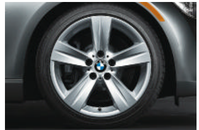
□ Star Spoke (Style 189) light alloy wheels and run-flat 1 performance tires. 2 In front: 18 x 8.0 wheels and 225/40 tires; in back: 18 x 8.5 wheels and 255/35 tires. (included in 335i Sport Package)
