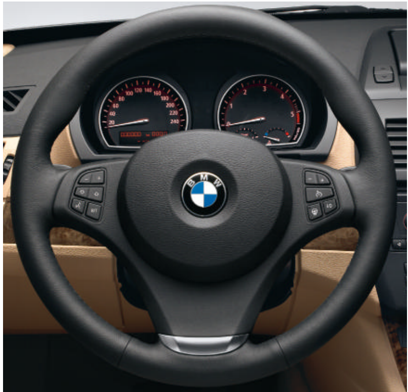
3-spoke leather-wrapped multi-function sport steering wheel offers controls for audio system, cruise control and (accessory) phone.
