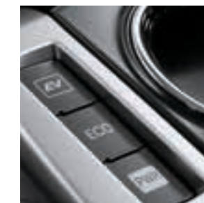
DRIVE MODE SELECT Different modes for different types of driving. ECO mode helps reduce fuel consumption. EV mode runs solely on battery power for up to 1.6 km under certain conditions. And Power mode increases gas pedal response for enhanced acceleration.
