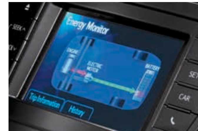
ENERGY MONITOR The Energy Monitor helps keep you continually apprised of the Hybrid Synergy Drive energy flow and how energy is efficiently managed and distributed.
