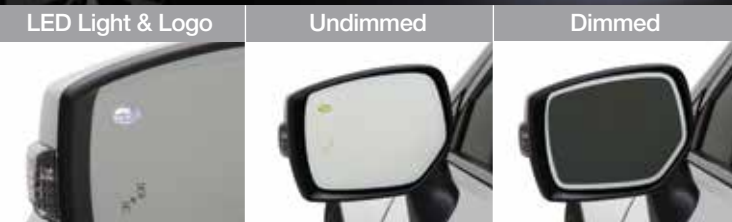
■ Exterior Auto-Dimming Mirror with Approach Light Enhance your Auto-Dimming Mirror experience by adding the Exterior Auto-Dimming Mirrors with Approach Light*. Open or unlock the doors with the keyless entry system and LED lights located behind the Subaru logo in each exterior mirror help to light the way. Light is cast down all four doors and onto the ground next to and towards the rear of the vehicle. When in traffic, the Exterior Auto-Dimming Mirrors help add to a safer driving experience by reducing headlight glare on the exterior mirrors. This occurs when excessive light is detected from the rear of the vehicle. The dimming level of the exterior mirrors is regulated by the level of light detected by the Interior Auto-Dimming Mirror. J201SAL001 J201SAL101 (with Blind Spot Detection)
