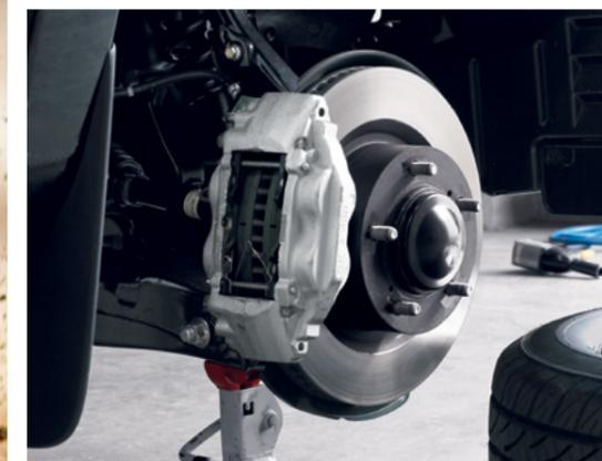
**POWERFUL BIG BRAKES** With big power comes big responsibility. That's why Tundra is equipped with enormous 13.9-in. front Brake Rotors and 4-piston calipers. Particularly when you're towing, Tundra's big rotors can help to provide the confidence that when you apply the brakes, the Tundra – and your trailer – will come safely to a stop.
