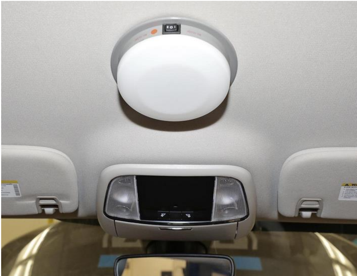
Figure 23: Police Dome Lamp (front shown)
