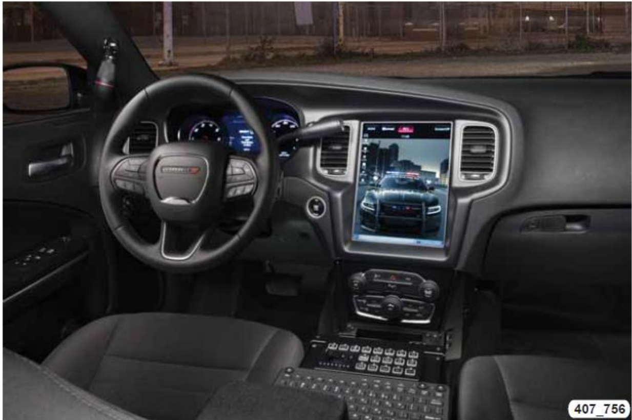
Figure 17: UConnect 12.1 System, aftermarket equipment shown
