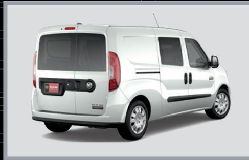
**OFFSET DOORS DESIGNED TO BE SIMPLER AND SAFER.** Positioning the larger of the two rear doors on the left gives you 10 percent greater access than typical 50/50 doors and lets you access the rear cargo area with greater confidence when traffic is adjacent. When the right side is open, there's less door width to move around.
