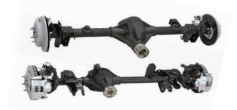
Front and rear axle assemblies will provide the next level of off-road performance for your CJ, YJ or TJ. These axles are shipped with current Wrangler Rubicon suspension mounting brackets installed. Adaptation of these units into previous models is the responsibility of the purchaser. These axles come completely assembled with 4.10 gear, and electric selectable locking differential.
