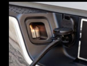
**BRIGHT LIGHTS. BIG TOWING.** Ideally positioned in the rear bumper well, the standard 4- and 7-pin trailer connector keeps the connections far from dirt and debris; adjacent illumination makes it a breeze to hitch or unhitch a trailer at night. Providing both pin settings eliminates the need for an adapter or jumper when hauling different trailer setups.
