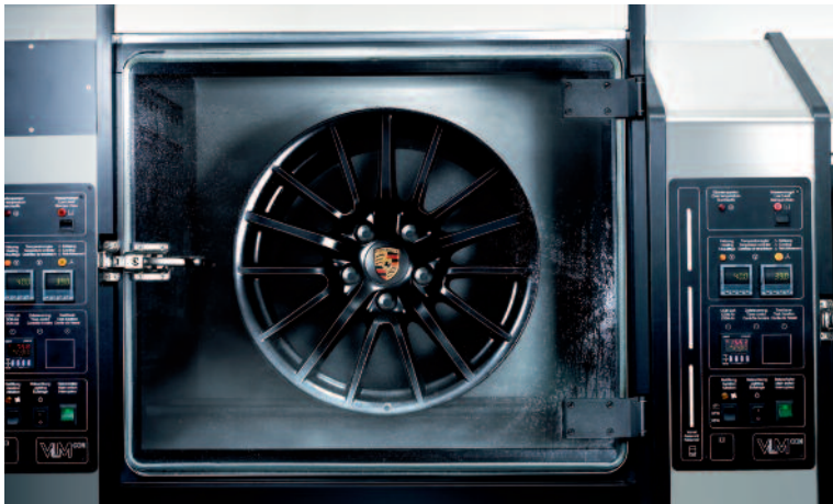
19-inch SportDesign wheel in a black high-gloss finish in the salt chamber
