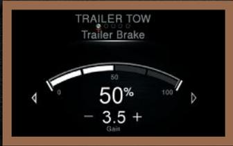
**Dozens of Menu Options** include data about the available trailer brake controller. This reading at left signals that the brake is at 50% of total operation with a 3.5% gain. You'll control the gain that's right for the terrain with the center stack-mounted trailer brake controller.
