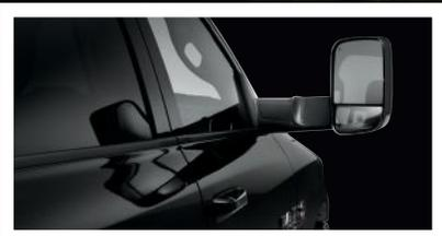
Monitoring your trailer is critical. Extra-wide available trailer-towing mirrors on each side are the answer. Measuring a substantial 7 x 11 inches, they offer a maximum view, with a wide-angle mirror monitoring peripheral traffic.
