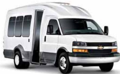
**COMMERCIAL CUTAWAY CHASSIS CAB** applications offer a choice of three wheelbases; wide B-pillars; and a full-length, ladder-type frame. See the back cover for information about alterations and warranties.
