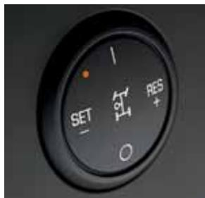
**POWER TAKEOFF (PTO) CAPABILITY<sup>1</sup>** allows HD Chassis Cab equipped with this GM segment-exclusive feature and the available Allison 1000 Series six-speed automatic transmission to power auxiliary equipment such as a dump body or hydraulic motors for generators or tools.
