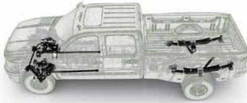
**OUR ALL-NEW CHASSIS FEATURES A HIGH-STRENGTH, FULLY BOXED STEEL FRAME**
