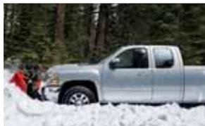
**EVERY HD 4x4 MODEL** can easily accommodate a snow plow with the available Snow Plow Prep Package, thanks in part to massive, forged, precision-machined upper control arms and a Front Gross Axle Weight Rating of up to 6,000 lbs.
