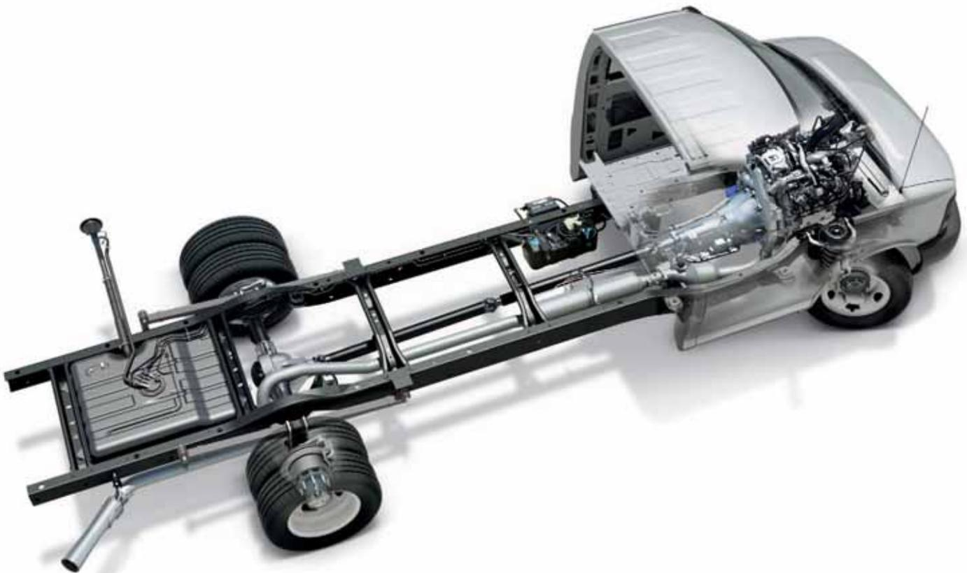
**EXPRESS 4500 CUTAWAY CHASSIS CAB.** The Express 4500 Cutaway offers a 159-inch wheelbase that is a perfect platform to take numerous upfits, including a school bus, ambulance, shuttle bus or recreational vehicle.
