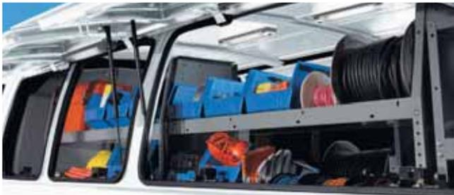
**AVAILABLE ACCESS PACKAGES** offer easy interior access to tools and cargo. Each includes three exterior, remote-release, side-access panels that can be opened by Remote Keyless Entry. Not available with optional driver-side 60/40 swing-out doors or sliding passenger-side door.
