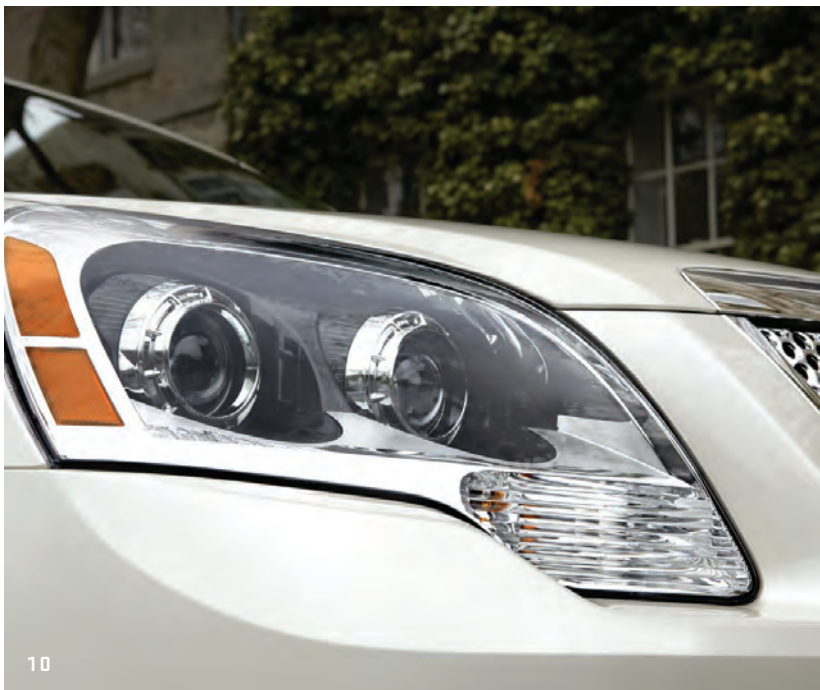
↓ Acadia Denali's standard High-Intensity Discharge headlamps provide a brighter, more focused light than conventional headlamps.
